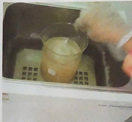
Fig 2.5: Beaker is placed in hot water bath at 80°C with continuous stirring.
