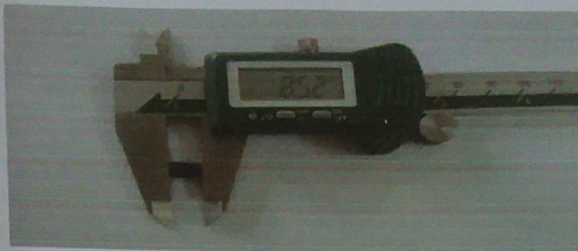
Fig-3.5.3: Photo of Measuring length of colour portion of Boring sample Then using following formula penetration(%) was calculated:
