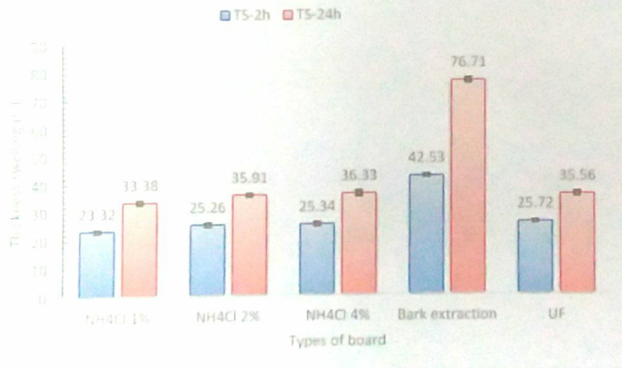
Fig. 7. Thickness swelling (%) of the boards after 2 and 24 hours of immersion in water
