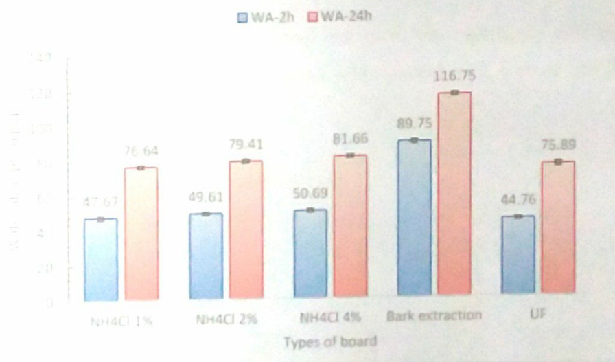
Fig. 6. Water absorption (%) of the boards after 2 and 24 hours of immersion in water
