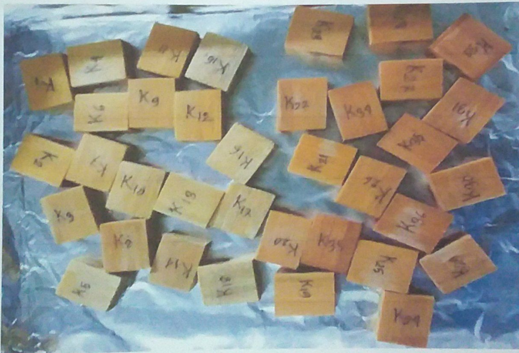
Figure 3: Wood samples after preservative treatment
