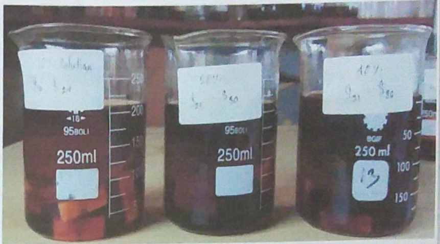
Figure 2: Vacuum treatment and preservative retention
