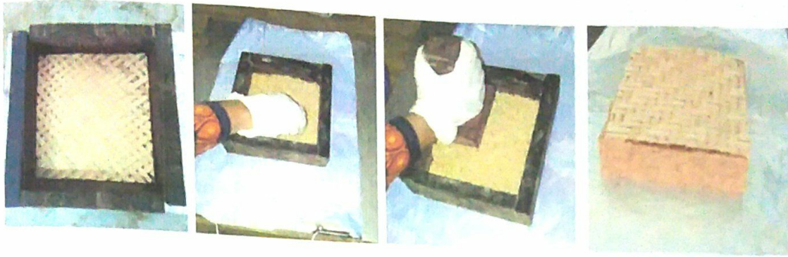
Fig: 3.4 Mat formation processes of bamboo mat board and particleboard
