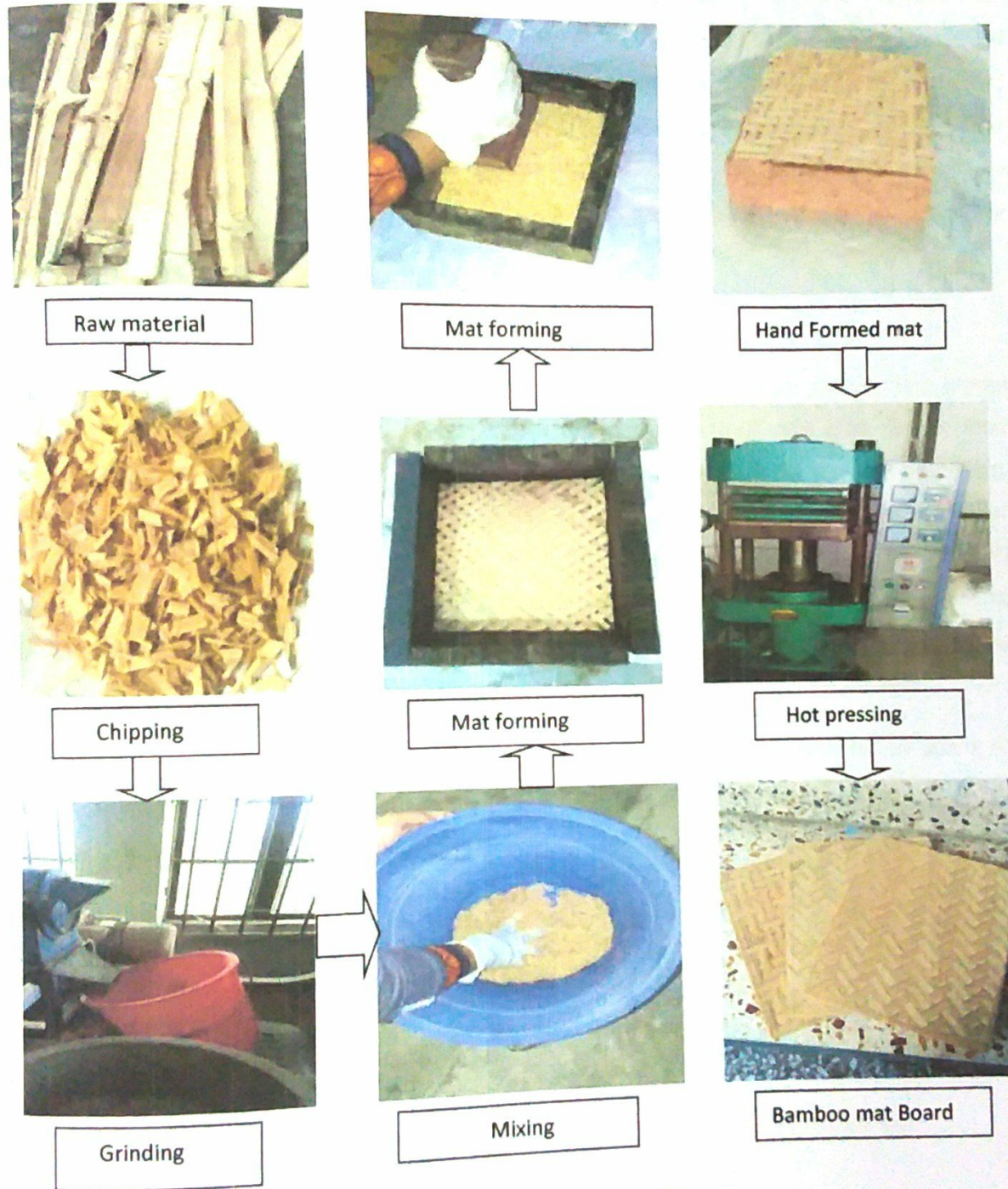
Fig: Manufacturing process of Bamboo mat Board
