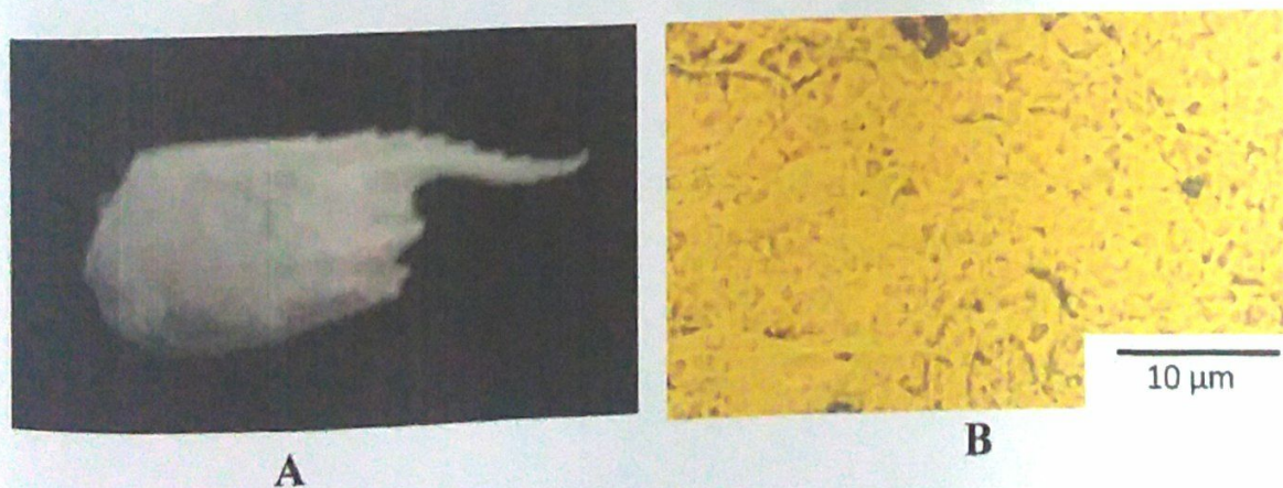
Figure 4.1. a) Semi transparent shrimp shell after chemical treatment. b) Microscopic view ( \times 40 ) showing homogenous dispersion of chitin nanofibers in acidic condition.
