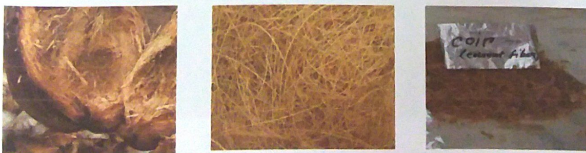
Figure 3.3: Processing of coir fiber
