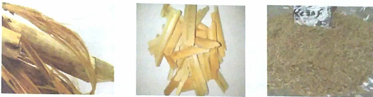
Figure 3.1: Processing and screening of kenaf particle
