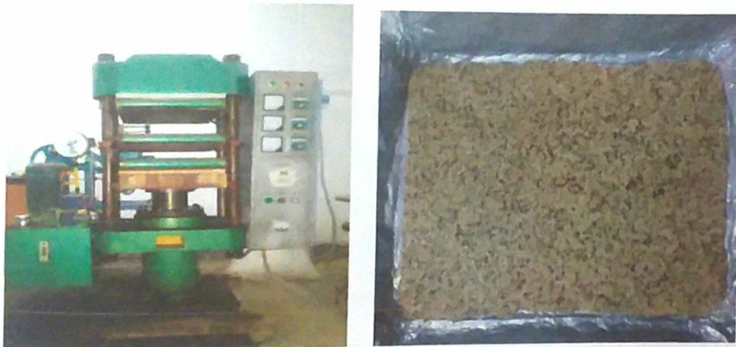
Figure 3.6: Hot pressing & board preparation
