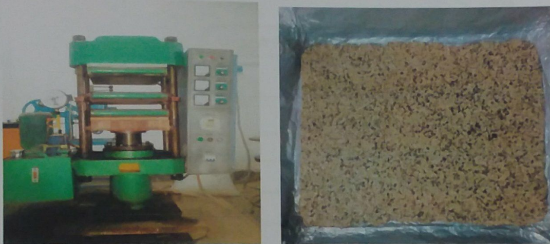
Figure 4: Hot pressing & board preparation
