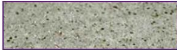
Fig. 4(a): Fibre cement board (FCB) is made of cement, water, fillers and fibres. The fibres may be synthetic (right) or natural
