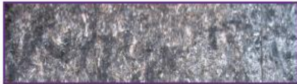
Fig. 4(c): Cement bonded particle board (CBPB) is made of cement, wood particles and water.
