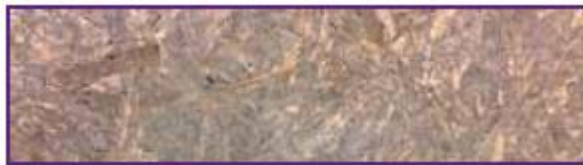
Fig. 4(d): Wood strand cement board (WSCB) is made of cement, water, salt and wood wool fibres. Density of 1100 kg/m 3
