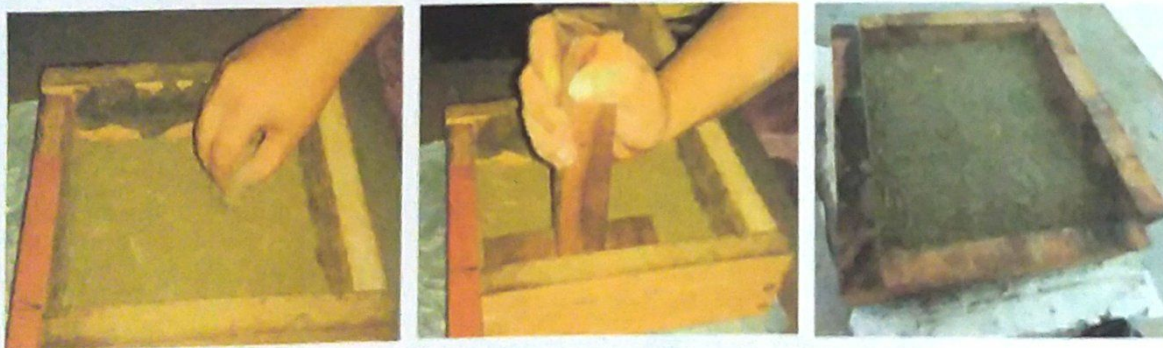
Fig: 3.17 Mat formation process of cement bonded fiber board
