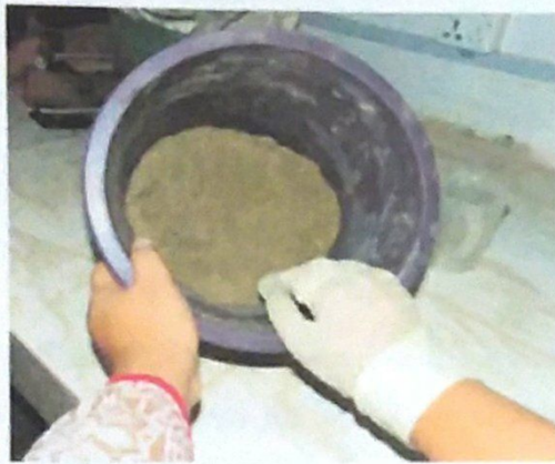
Fig: 3.16 Mixing of fiber, cement and water
