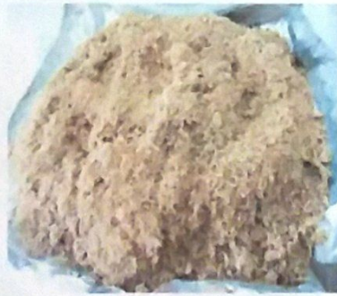
Fig: 3.8 Hot Water Treated Fiber
