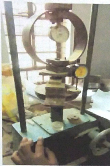
Fig: 3.23 Mechanical testing of CBF
