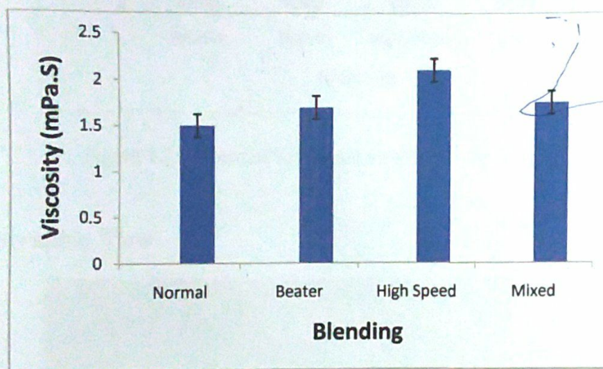
Figure 4.1 Viscosity of pulp at different blending revolution
