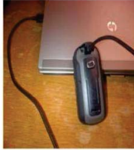
Figure b: Connect the USB cable with GPS device
