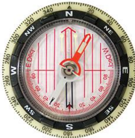
FIGURE 5: THE BEARING MEASUREMENTS ARE NUMBERED AROUND THE OUTSIDE OF THE INSTRUMENT.
