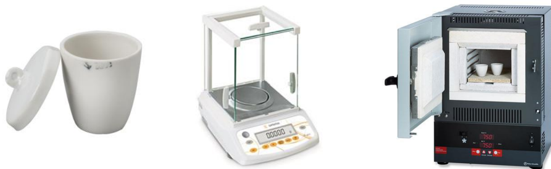
Figure 4: Porcelain cup, high precision analytical balance and muffle furnace
