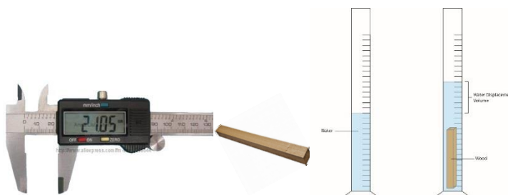
Figure 3: Measurement of wood volume using water displacement method
