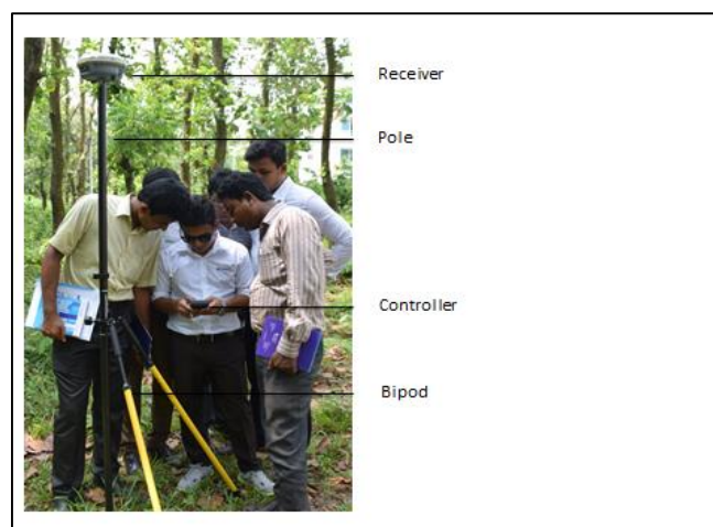
Figure 3: Rover installation and positioning
