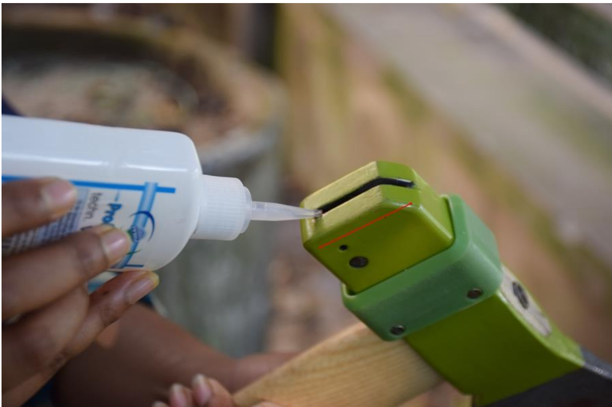
Figure 43: step 2- Putting Vaseline in the axe
