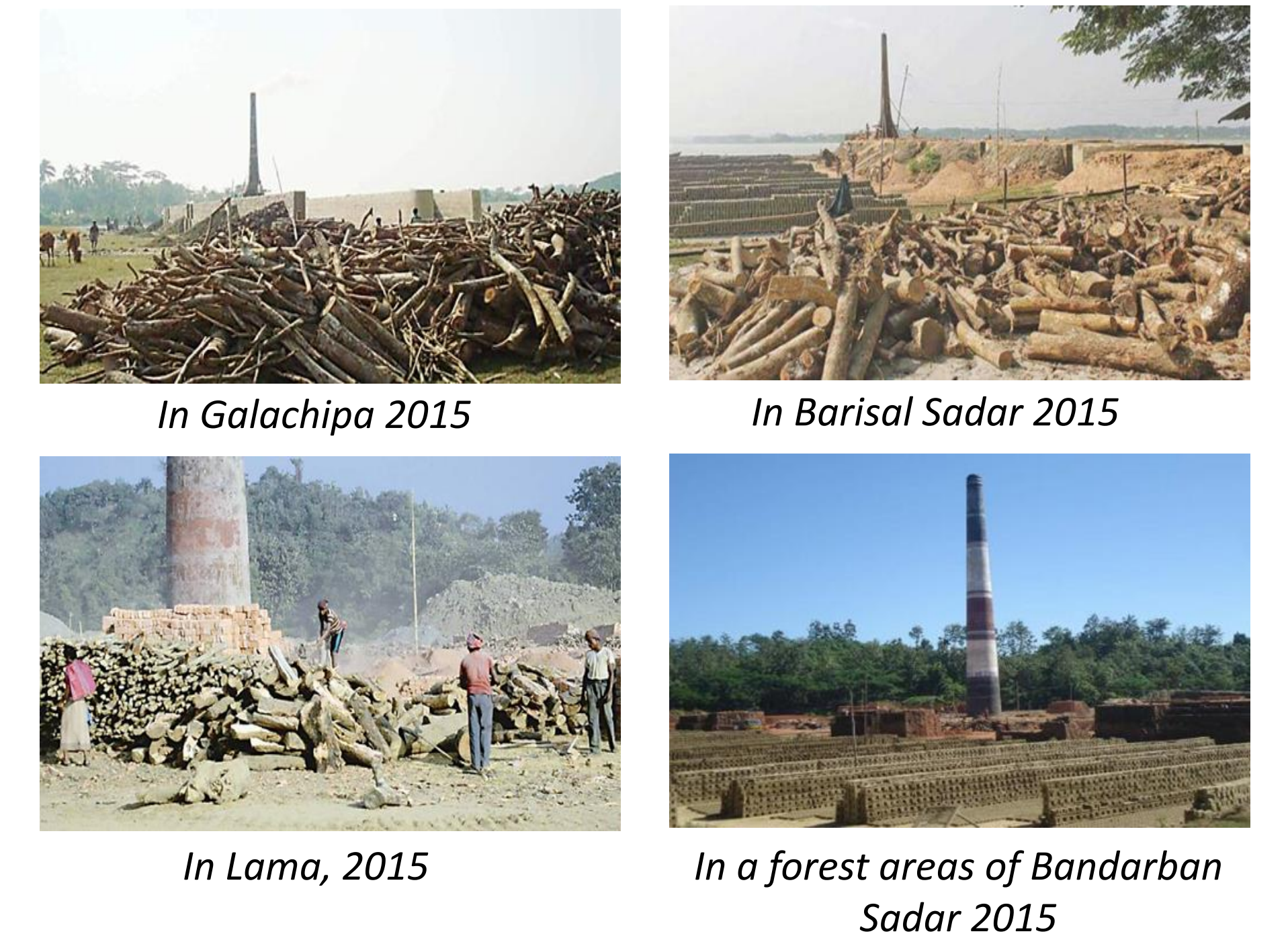
Figure 2: Fixed chimney kiln using fuel wood (source: The Daily Star)
