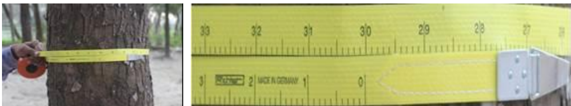
Figure 3: Diameter measurement procedure using diameter tape
